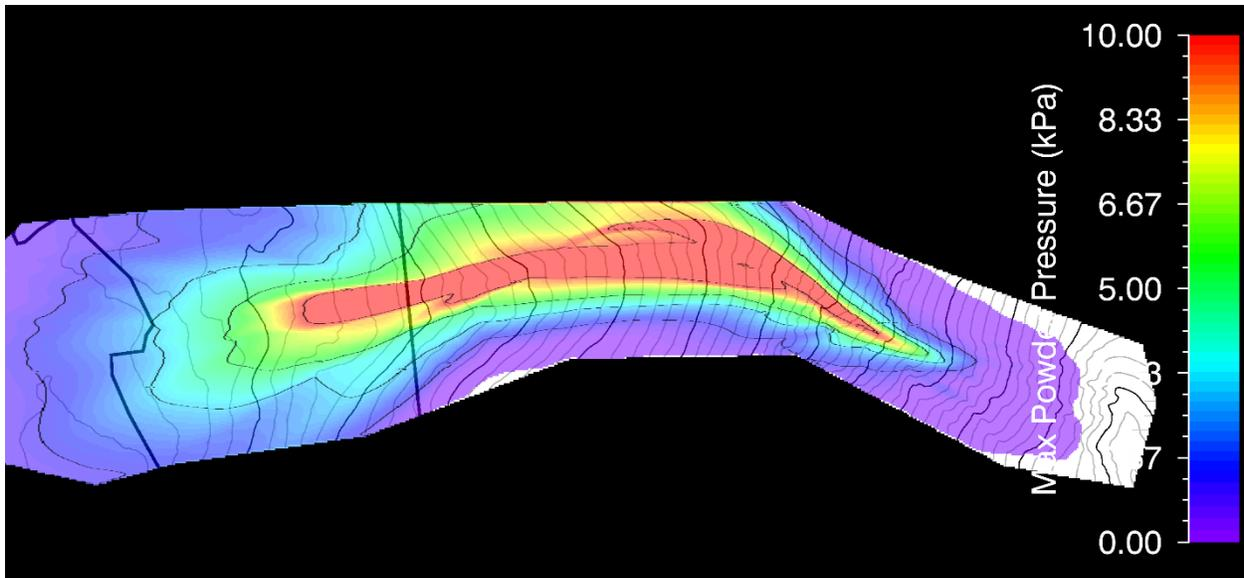
Figure 14 – Bavarian Path Powder Pressure from RAMMS:Extended Model
