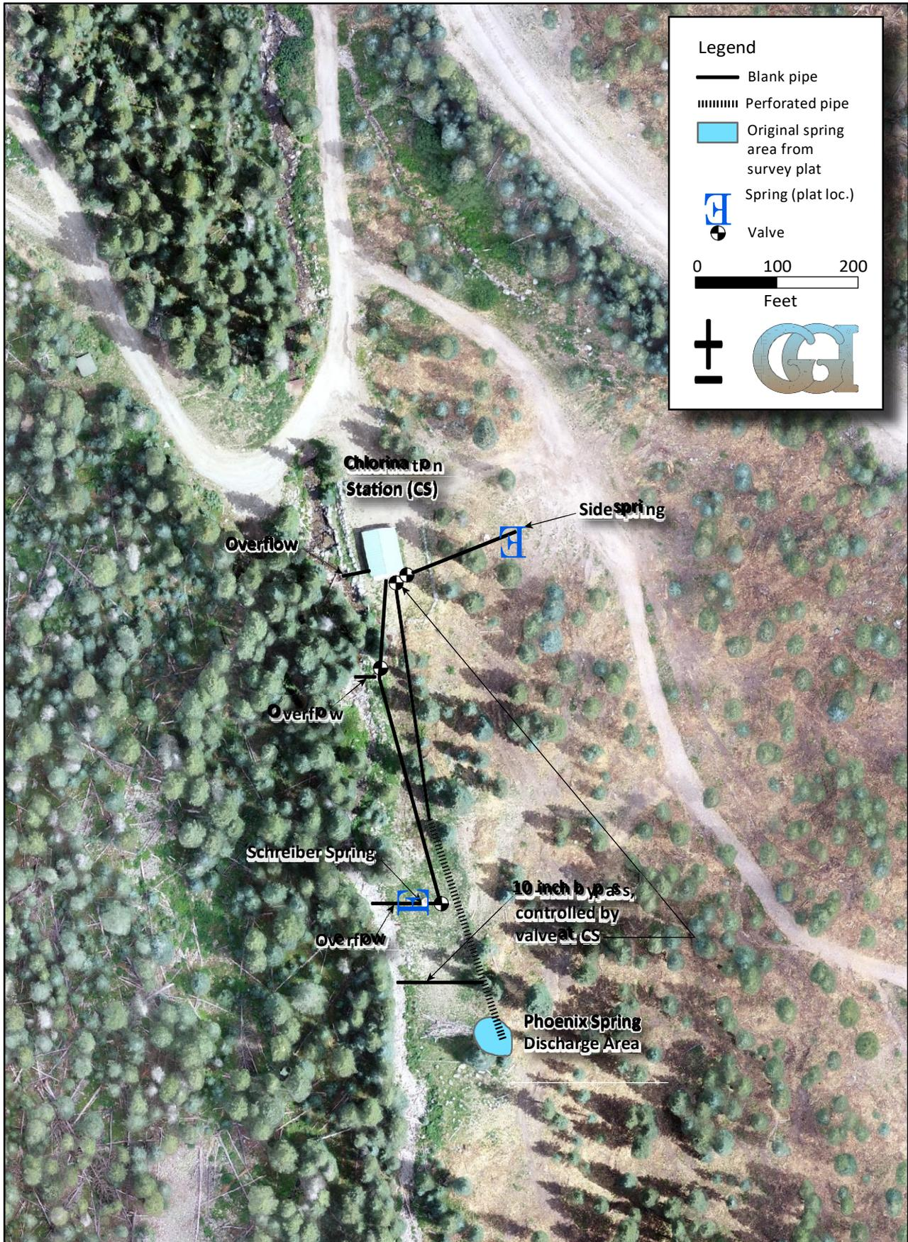
**Figure 2.** Schematic overview of spring flow collection and control system. Reconstructed from survey plats made prior to chlorination station construction and from schematic drawings of valve controls from VTSV staff (see Appendix C).
