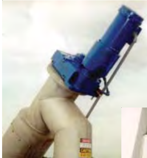
The Raptor Micro Strainer's enclosed drive assembly reduces maintenance expenses.
