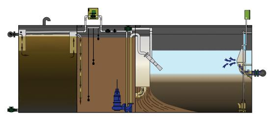
**Filled Decant Phase:** If, during peak flow events, the SAM<sup>™</sup> reactor reaches TWL before the decant phase ends, influent flows in a reverse direction through the surge return line and overflows the surge chamber secondary weir, and is diffused into the settled sludge at very low velocity as the decant phase continues.
