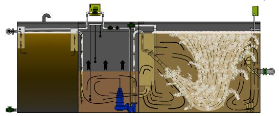
**Interact Phase:** When the level in the SBR reaches TWL, nitrified mixed liquor overflows the surge chamber weir and is returned to the SAM<sup>™</sup> chamber to mix and react with the raw influent. Aeration is cycled on and off to provide the required oxygen. Denitrification is reliable and complete. Scum is also removed from the SBR basin.
