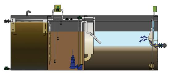
**Decant Phase:** When the settle timer expires, the decant valve is opened, and treated effluent is withdrawn from the upper portion of the SBR basin by means of a fixed solids excluding decanter.
