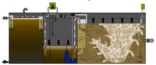
**Fill Phase:** When the level in the SAM<sup>™</sup> reactor reaches a predetermined "control level" the motive liquid pump is started. The SBR basin is filled and mixed. A percentage of the pumped flow is returned to the anaerobic chamber where biological solids settle. The recycle flow is adjustable to maintain the desired MLSS concentration in the SBR basin. Settled solids in the anaerobic chamber are digested.
