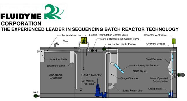
**System Components:** Influent continuously enters the anaerobic chamber where solids settle. Settleable BOD is converted to soluble BOD. BOD is reduced by 30%, and solids are reduced by 60%. The influent then flows to the SAM<sup>™</sup> reactor. Mixed liquor is maintained in the SAM<sup>™</sup> reactor to suppress odors, and initiate and accelerate carbon and nitrogen reduction.
