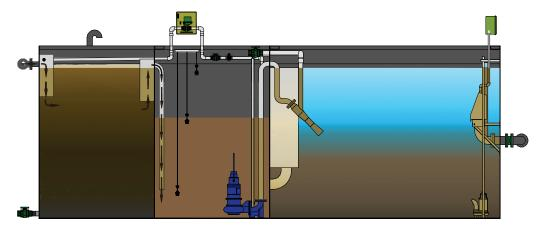
**Settle Phase:** When the level in the SAM<sup>™</sup> reactor again reaches "control level," aeration is discontinued, and the SBR basin settles under perfect quiescent conditions.
