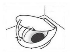
Keep lid closed at all times when the toilet is not in use to insure the primary air flow is through the exterior inlet vents.
