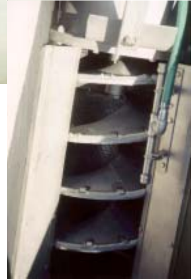
The stainless steel, shaftless screw conveyor improves screening performance.
